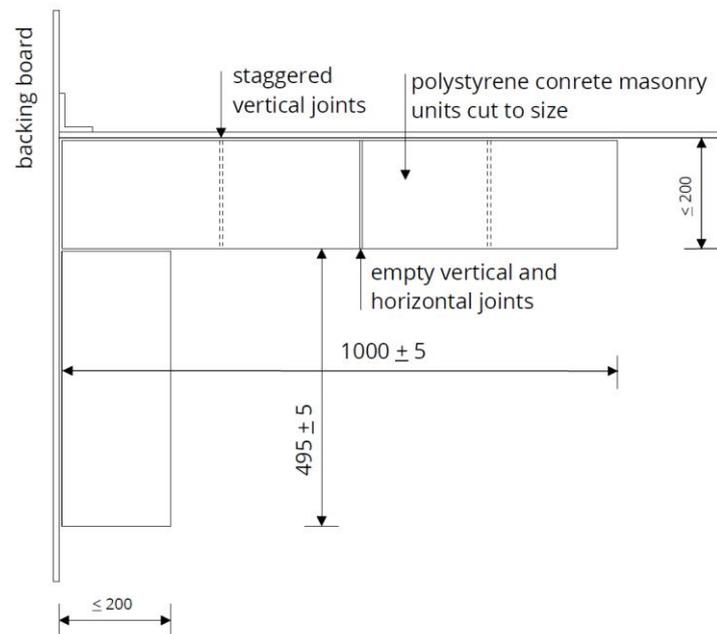
Figure D.1 Test rig configuration for polystyrene concrete masonry units
