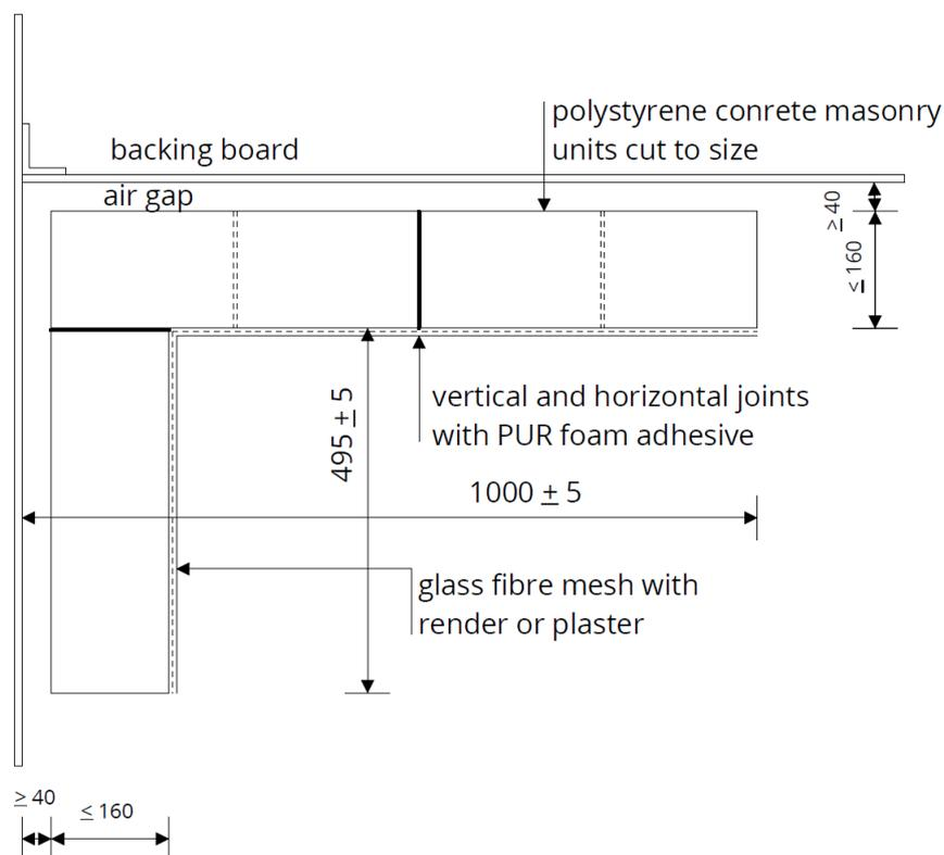
Figure D.2 Test rig configuration for the wall kit
