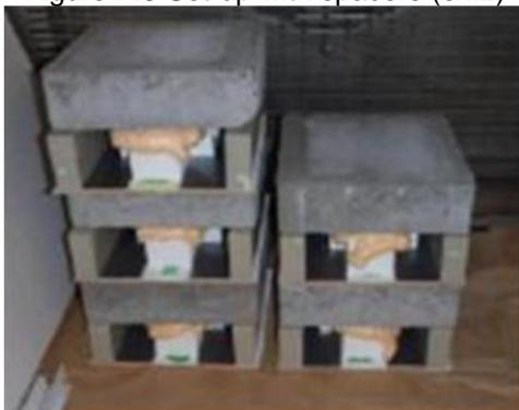
Figure F.5 Test sample during curing (48hrs)
