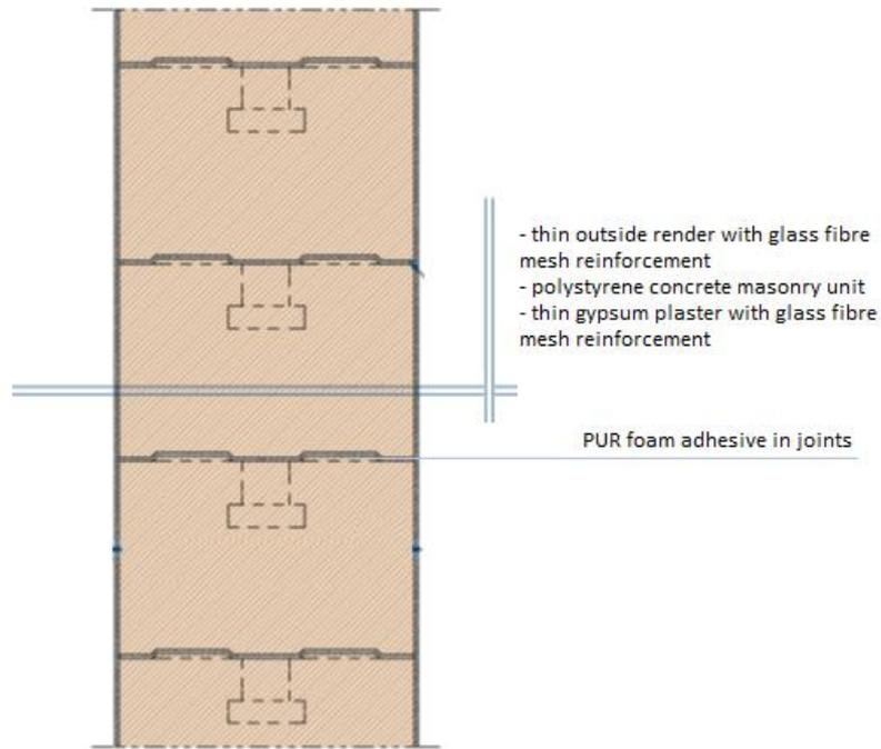
Example vertical section of an assembled external wall
