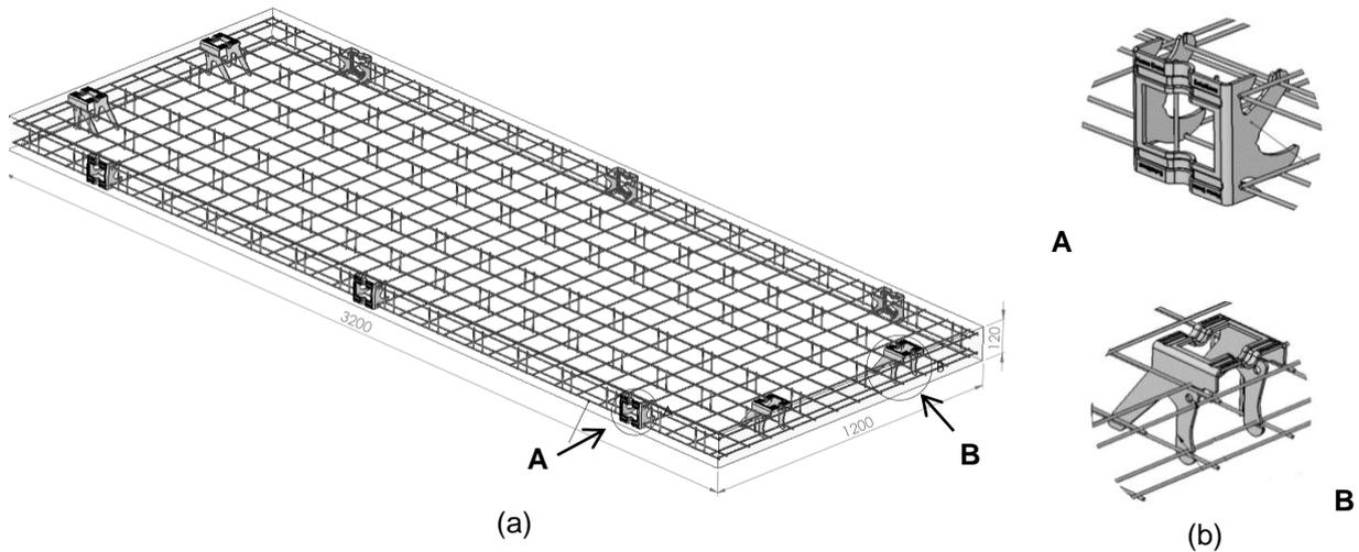
Figure 1.1 - (a) Loadbearing panels and particular of the fixing brackets: (b) “A” system and “B” system
