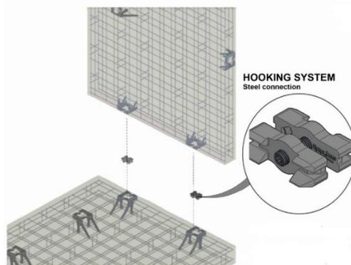
Figure 1.2 - Particular of the hooking system
