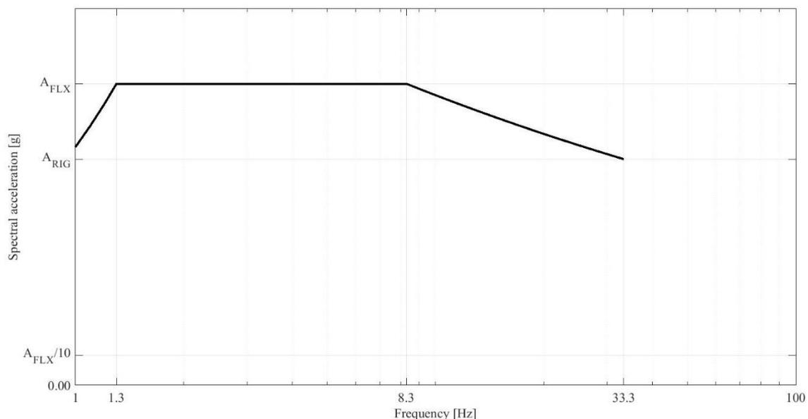
Figure E.5 - Required response spectrum (RRS), 5% damping
