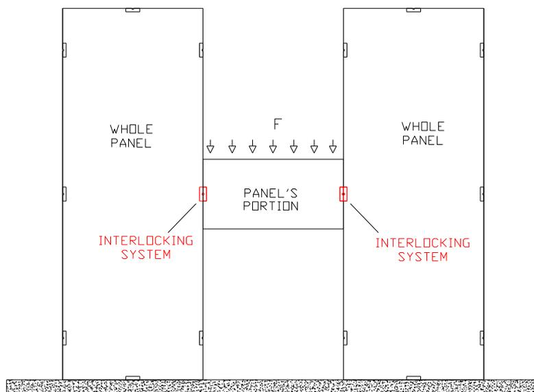
Figure D.4 - Example of shear tests assembly
