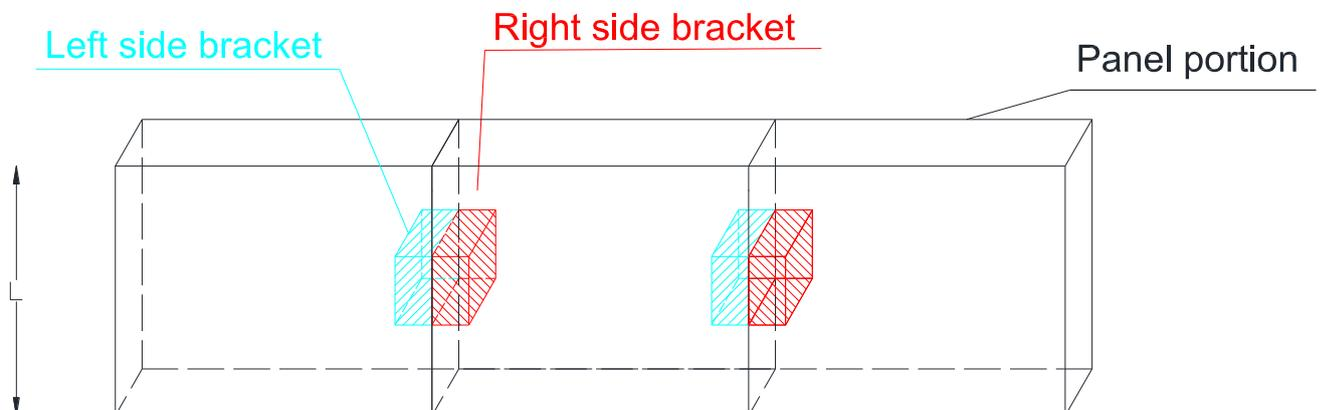
Figure D.2 - Example of test specimen for shear tests of the joint between panels
