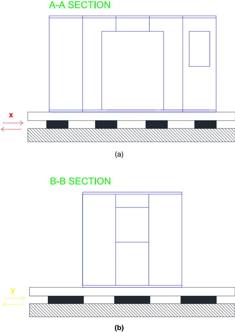
Figure E.3 - Lateral view of the test setup in (a) x and (b) y direction
