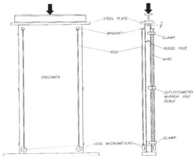
Figure B.1 - Setup for axial load test
