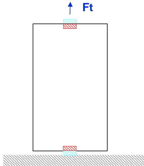
Figure D.3 - Example of tensile tests assembly
