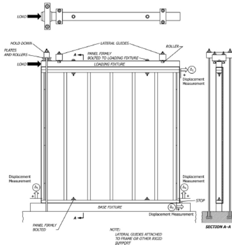
Figure C.1 - Setup for racking load test
