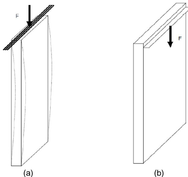
Figure 2.1 - Schematic view of panel subject to (a) axial loads and (b) eccentric axial load
