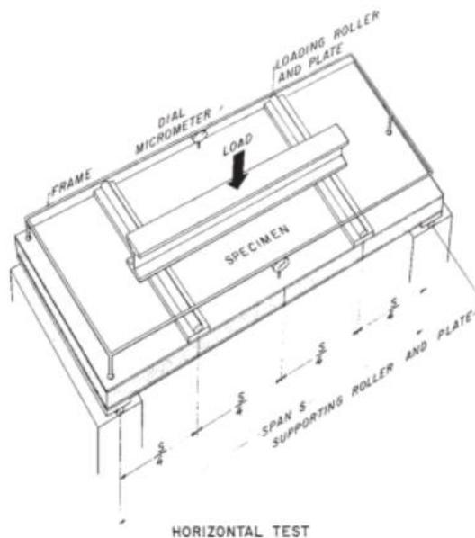
Figure A.1 - Setup for flexural test
