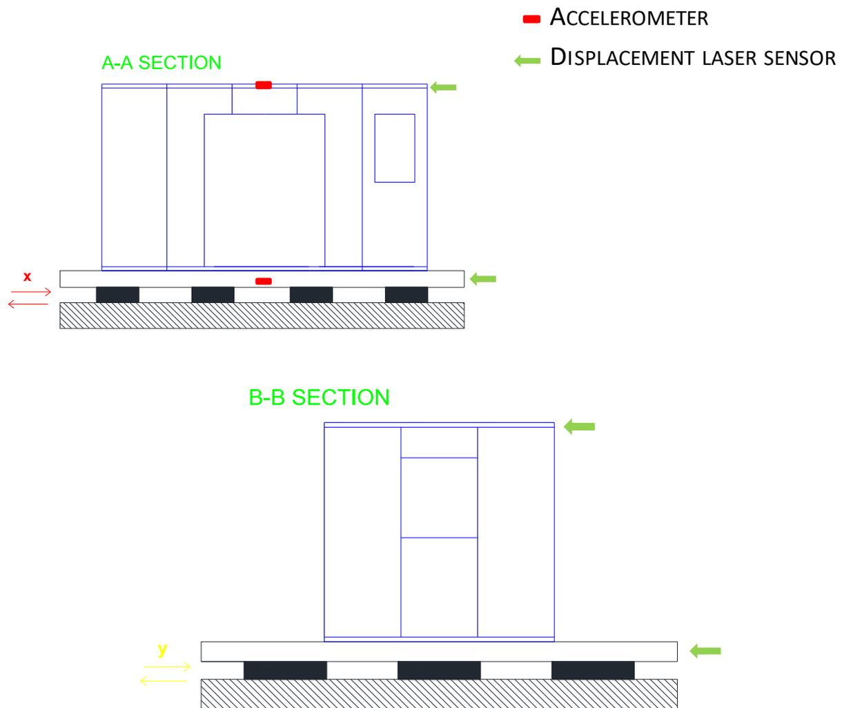
Figure E.4 - Example of specimen monitoring system
