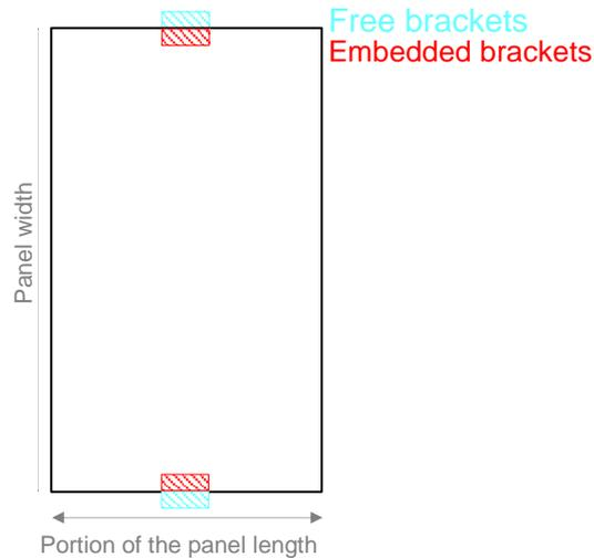
Figure D.1 - Example of test specimen for tensile tests of the joint between panels
