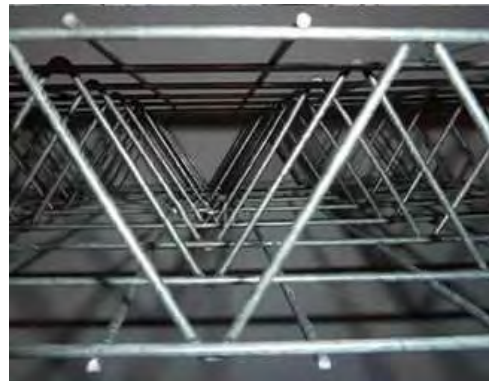
Fig 1.3: Welded reinforcing mesh 3-D panel without expanded polystyrene core.
